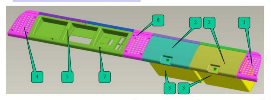
The installation principle is to install from the two sides to the middle, First installment 1 and 4, and finally mount 6.
